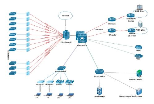
Hardware component summary 2 x Cisco Catalyst WS-C6509-E Switches 50 x WS-C2960XR-48FPS-I Switches 50 x CR50iNG Firewall
